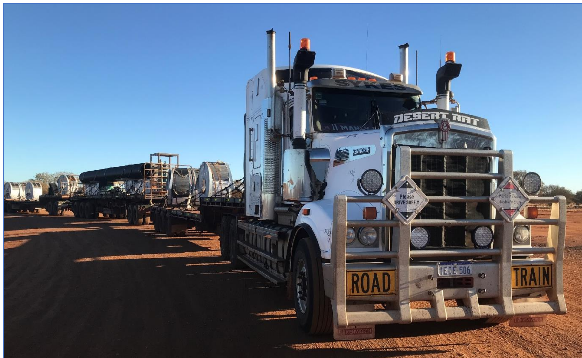
Kenworth 909 triple I took to PH, 53.5 meters long, 600 Horsepower
